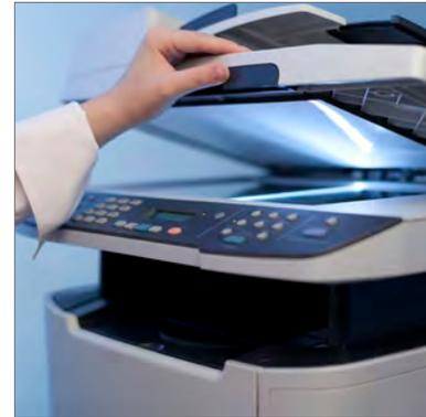
Multifunction printers or office copy machines are used as scanners in large offices. They allow an image of a scanned document to be emailed from the machine to a selected recipient. Organisations that have specialised scanning needs, such as the need to scan large maps or high volume batch scanning, will seek out different scanning solutions.
